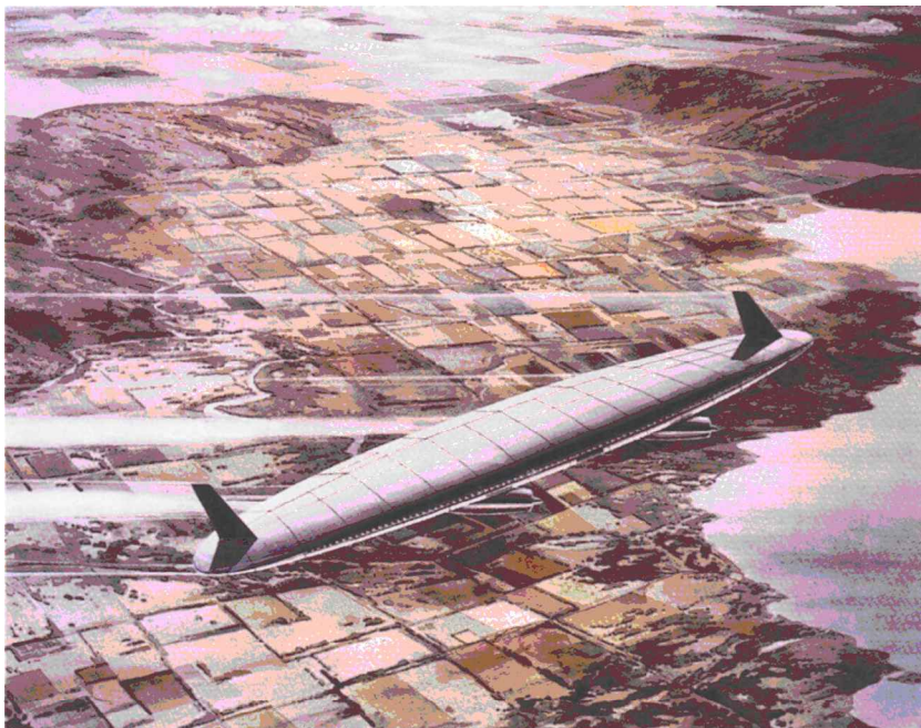
Fig. 1 NASA artist's concept of R. T. Jones' oblique wing supersonic transport.
